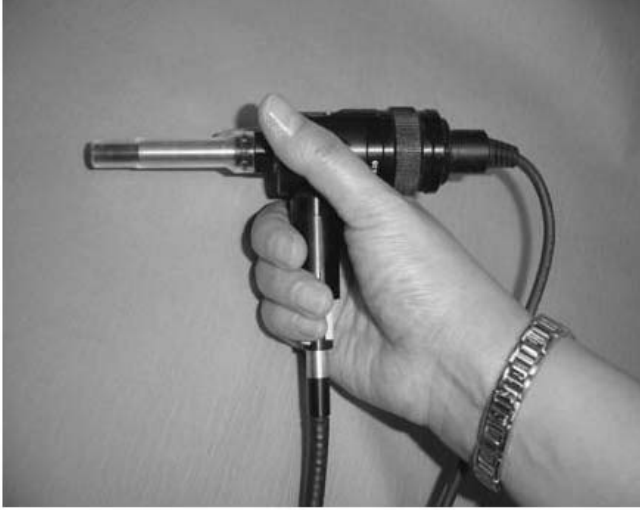
Fig. 2. Orthogonal Polarization Spectral imaging camera: CYTOSCAN A/R (Cytometrics Inc., Philadelphia, PA).
