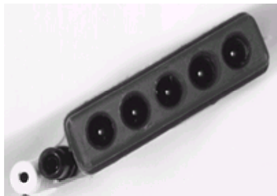
Figure 8-35. The current standard for patient lead wires ( left ) requires a female connector. The patient cable ( right ) has shielded connector pins that the lead wires plug into.
