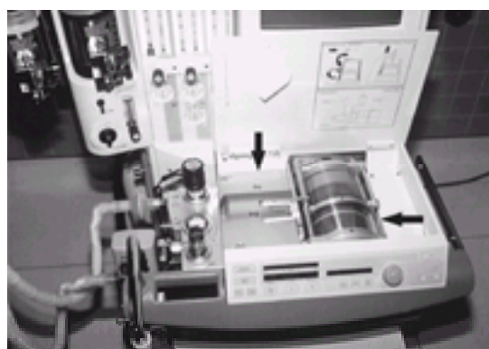
Figure 22-26. The Narkomed 6000. The horizontal arrow indicates the piston cylinder unit. The vertical arrow indicates a rectangular manifold that houses the valves for fresh gas decoupling.
